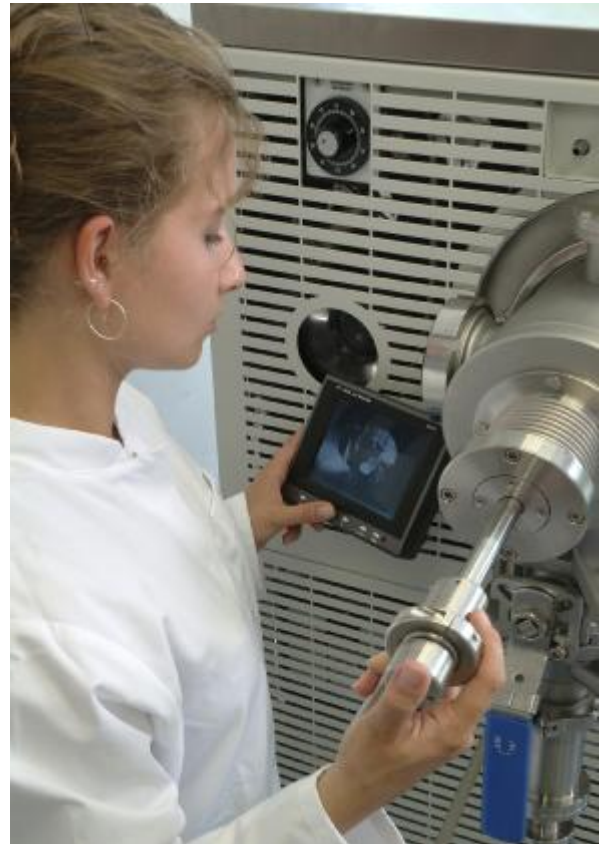
Example: sample thief/manipulator with camera monitoring
