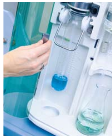
Protective door monitored by a sensor
