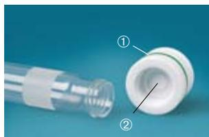
Colored O-rings used to label different adapters. Porous PE frits for foam and splash protection, e.g. for sample adsorption onto silica.
