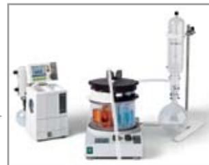
Comprehensive solution for automatic distillation, sophisticated vacuum control with pressure profiles, repeat function, sec. condenser and much more...
