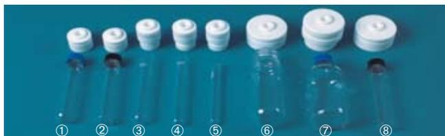
Selection of sample tubes with their corresponding adapters. The full range is listed in the Adapter Guide. A set of seals is included in the adapter set. Further seals are recommended as spare part.
