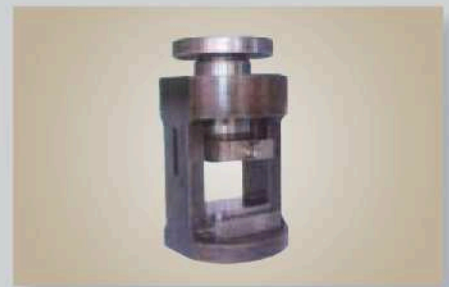
Concrete test attachment
