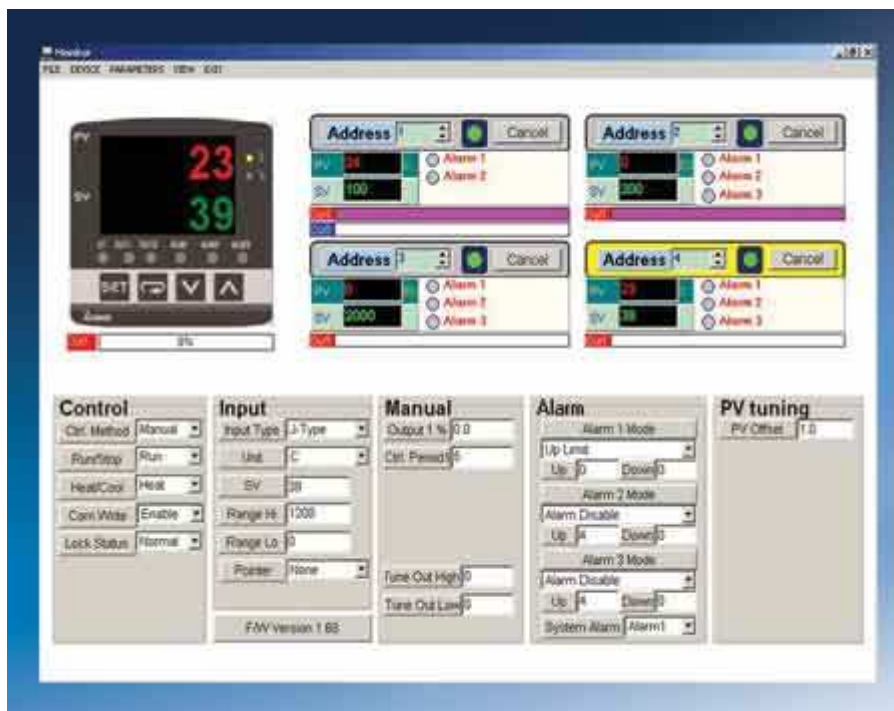
Screenshot from remote PC showing Set Point and Process values for up to four variables. Lower section showing operating parameters of active module.
