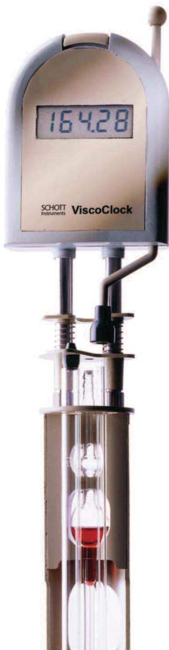
For temperature stabilization in the thermostatic bath, the following tempering liquids are suitable: water, alcohol water (e.g. ethanol, methanol), paraffin oil, and silicone oil. Liquids can be measured that qualify for use with the viscometer being used in each instance.
