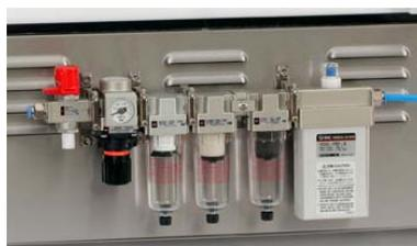
A constant flow acc. to the standards can be set with a built in flow meter.
