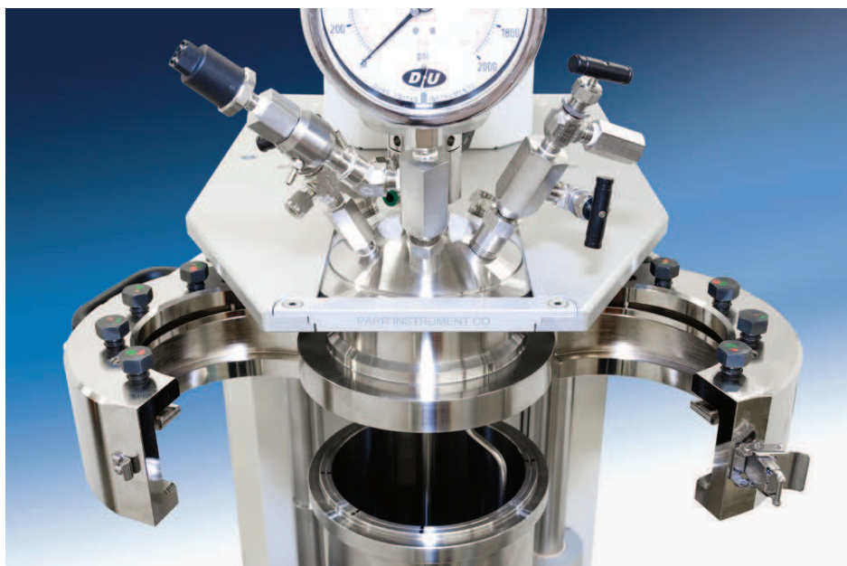
The innovative Parr Hinged Split-Rings on the 4553 and 4554 add to a safe vessel removal routine. Simply loosen the compression bolts, unlatch the split-ring closures, and pivot the split-rings out of the way.
