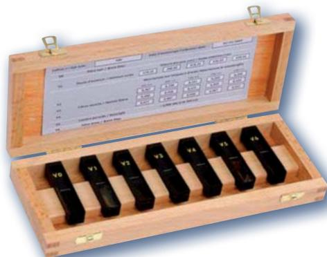
*Performance validation kit with filters and software. Every Uvikon comes fully tested and includes a factory Certificate of Performance. All test data is archived at the factory for full traceability*
