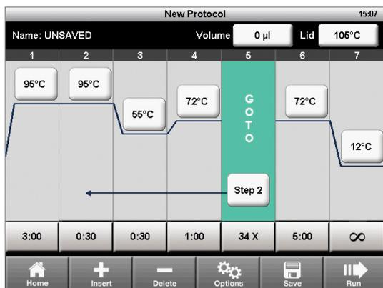
**Intuitive graphical programming.** The thermal cycler's onboard software displays an editable thermal profile of the PCR protocol, making it easy to create and run new protocols.
