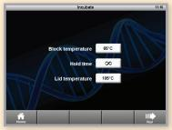
Incubate instantly. The convenient incubate feature keeps your samples at a constant temperature for ligations or restriction digests.
