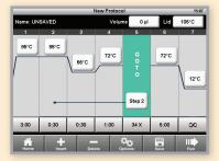
Create a new protocol in just seconds. The protocol editor displays the thermal profile in an intuitive, graphical format.
