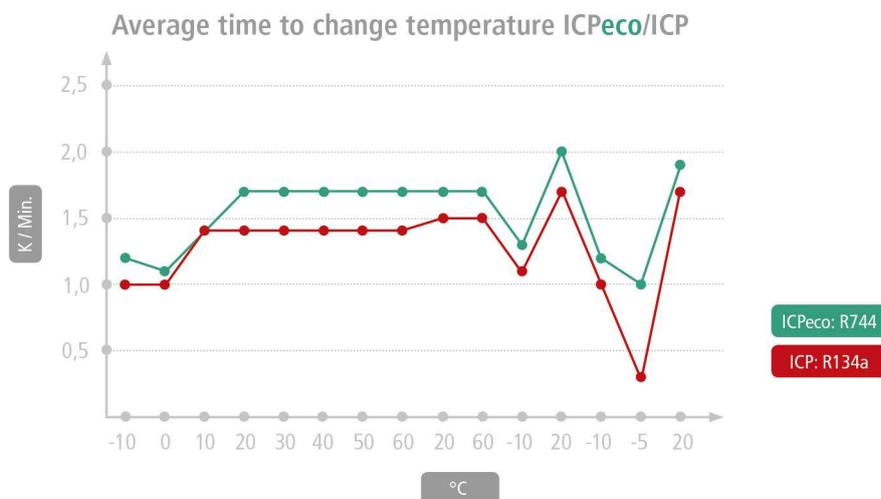
On average 20 % faster temperature change rates with a CO<sub>2</sub>-cooled compressor (measurement ICP260eco at ambient temperature +22 °C according to IEC 60068-3-5)
