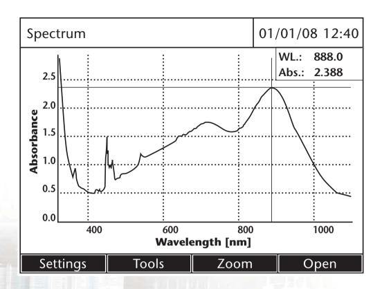
Whenever the optimal wavelength for the determination of the concentration is unknown or the purity of a solution is to be determined, the adding of a **spectrum** becomes necessary. By using the zoom function and the cursor it is quite easy to edit the spectra.
