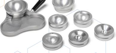
The largest sized insert you use in parallel will determine the DrySyn base plate you'll need!
