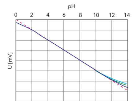
6 Exemplary mV curve of various electrode for different pH values. Legend: --- Ideal characteristic; — Real characteristic for electrode 1; — Real characteristic for electrode 2; — Real characteristic for electrode 3
