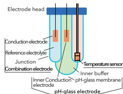
1 Structure of a single rod measuring cell
