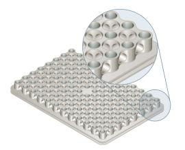
Bio-Rad's patented reduced-mass sample block heats and cools more quickly than standard blocks, improving thermal uniformity and minimizing edge effects.
