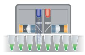
As the CFX Opus Systems' optics shuttle travels across the plate, light is focused into the center of each sample well. Side view of the optics shuttle shows the 450–490 nm LED firing and SYBR® Green emitting at 520 nm into the detector.
