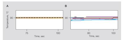
**Superior thermal uniformity for reproducible results.** The temperature measured by probes in 15 wells across a sample block. **A**, temperatures across the sample block vary by ±0.3°C for the CFX Opus 96 and 384 Systems, an improvement of 0.1°C over **B**, the temperature variability across the CFX Touch Systems' sample block.
