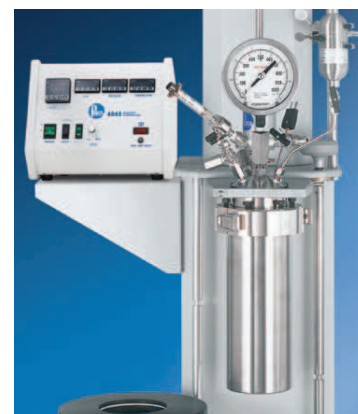
4534 Reactor, assembled with heater down.
