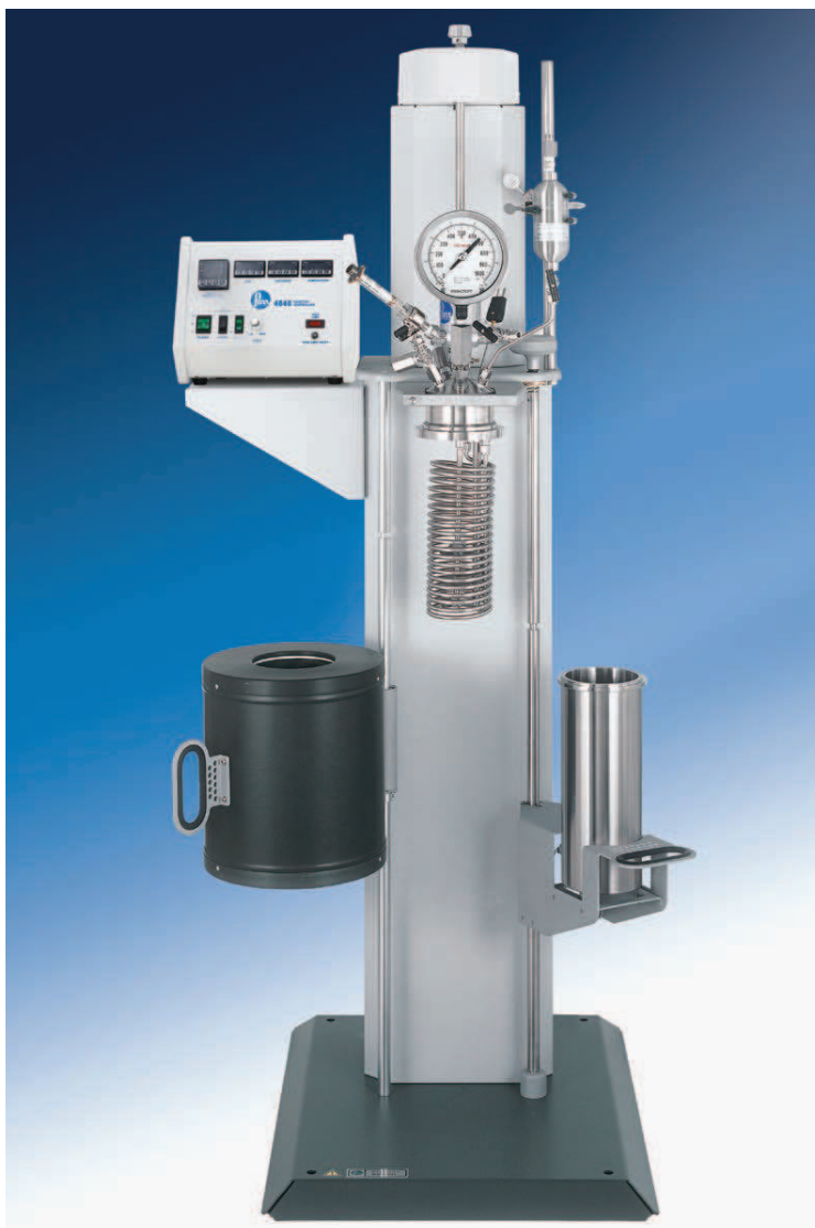
4534 Floor Stand Reactor, 2000 mL, Fixed Head, with Spiral Cooling Coil and Liquid Charging Pipette, in the open position, and a 4848 Controller with optional Expansion Modules.
