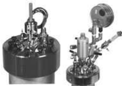
Multiple Electric Leads on the Head of a Pressure Vessel 2000 mL Bomb Head Assembly with Pressure Relief Valve and Transducer
