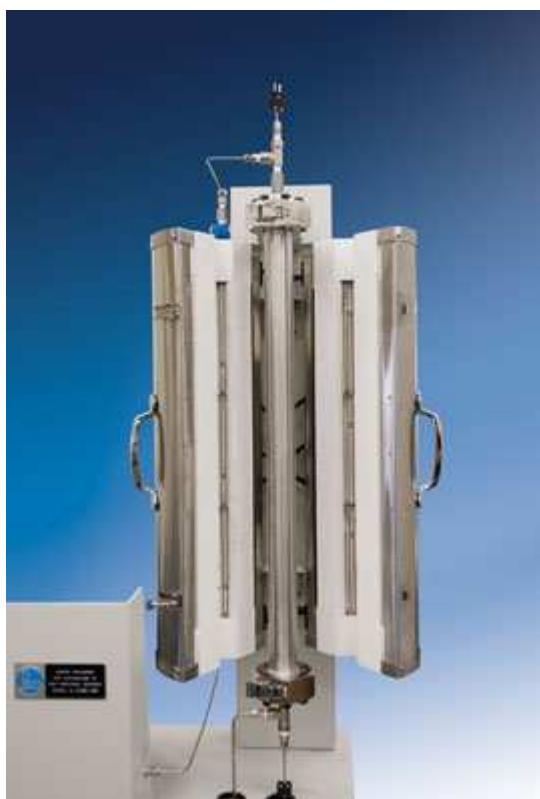
3-Zone Split Tube Furnace with 1" Tubular Reactor
