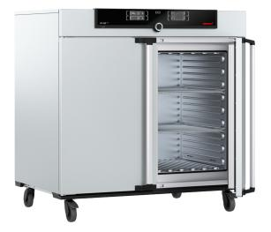
The universally applicable lab oven U is Memmert's classic appliance for temperature control in science, research and material tests in industry. The technologically perfected masterpiece made of high-quality, hygienic, easy-to-clean stainless steel leaves nothing to be desired in terms of ventilation and control technology, overtemperature protection and precisely tuned heating technology.
