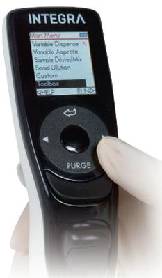
A choice of ten predefined pipetting modes provides users with convenient solutions for the most common liquid handling tasks. Standard pipetting routines, such as repeat dispensing or serial dilutions can be executed with minimal set up time.
