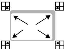
Move the tip rack to one corner, e.g. to the front left to load the back right quadrant. Hold the **Control unit** (6) and lower the pipetting unit down onto the tip rack and load tips by pressing **OK**.
