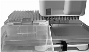
Place a rack on either the left or right position, and slide the two position stage to underneath the pipetting unit to correspond to the desired number of columns loaded.
