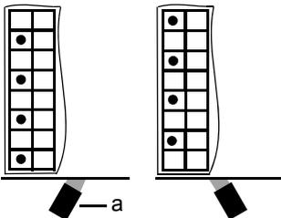
**Slider left:** pipette the front positions of a 384 well plate, sliding of 24 columns is guided.
