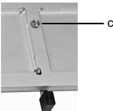
The Two position stage can be moved step by step sideways, corresponding to the 12 columns of a 96 or 24 columns of 384 well plate, respectively.
