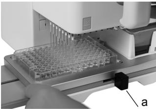
Move the **Stage slider** (a) to the middle to pipette 96 well plates.
