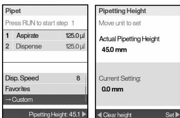
With tips attached move the **Pipetting unit** down to the desired pipetting height.
