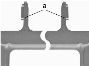
If it is noticed that the **Second stage** is not level, use a 1.27 hexagon screwdriver and tighten or loosen the two screws (a) on the stage the same amount, to ensure that both sides are the same height.
