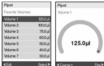
Move finger on the **Touch wheel** to choose (and highlight) an option on the display. Press **OK** (16) to make the selection.
