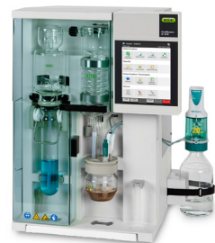
KjelMaster K-375 Steam distillation and titration
